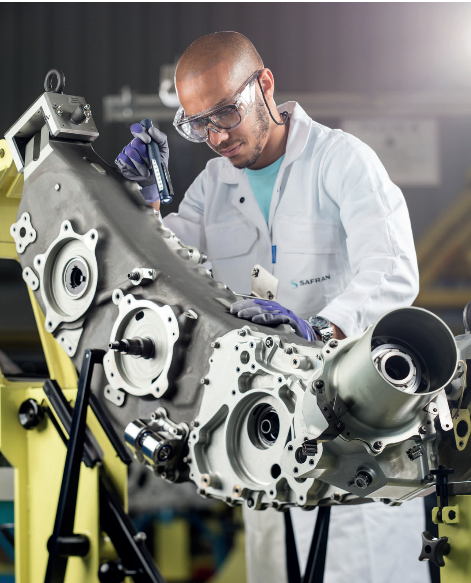
LEAP 1-B AGB (Accessory GearBox) quality control
