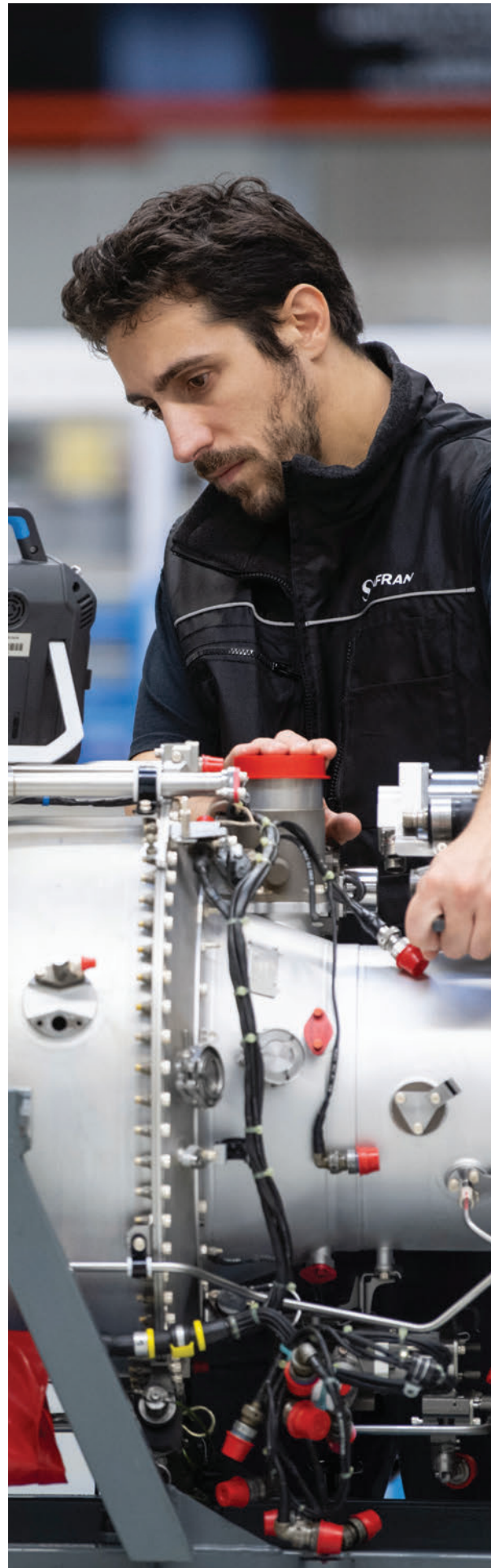
1. Detail of the LEAP-1A fan casing on the rolling line 2. Endoscopic inspection and parts inventory on a Makila engine
