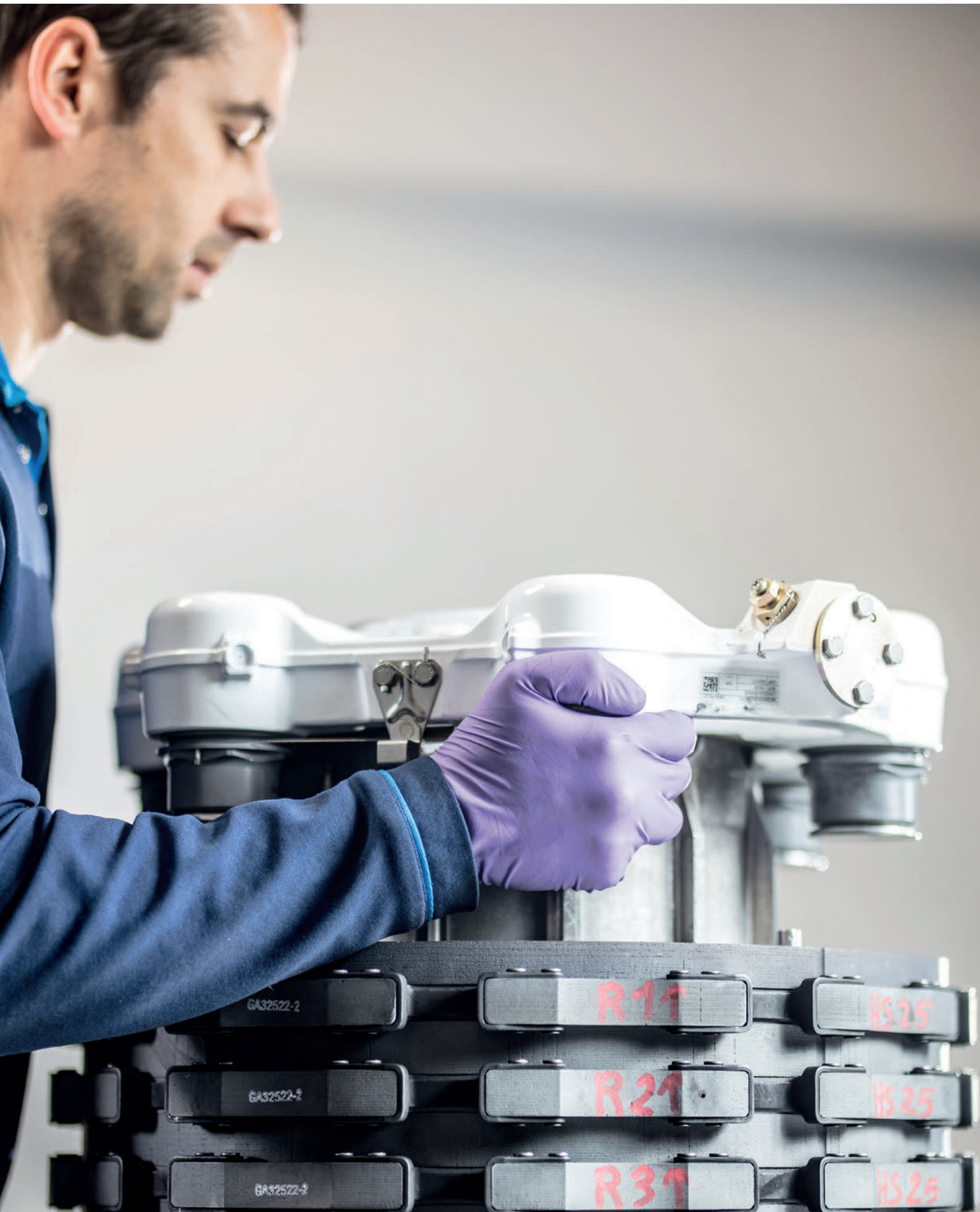
Assembling the carbon discs for the brake system on the 777X
