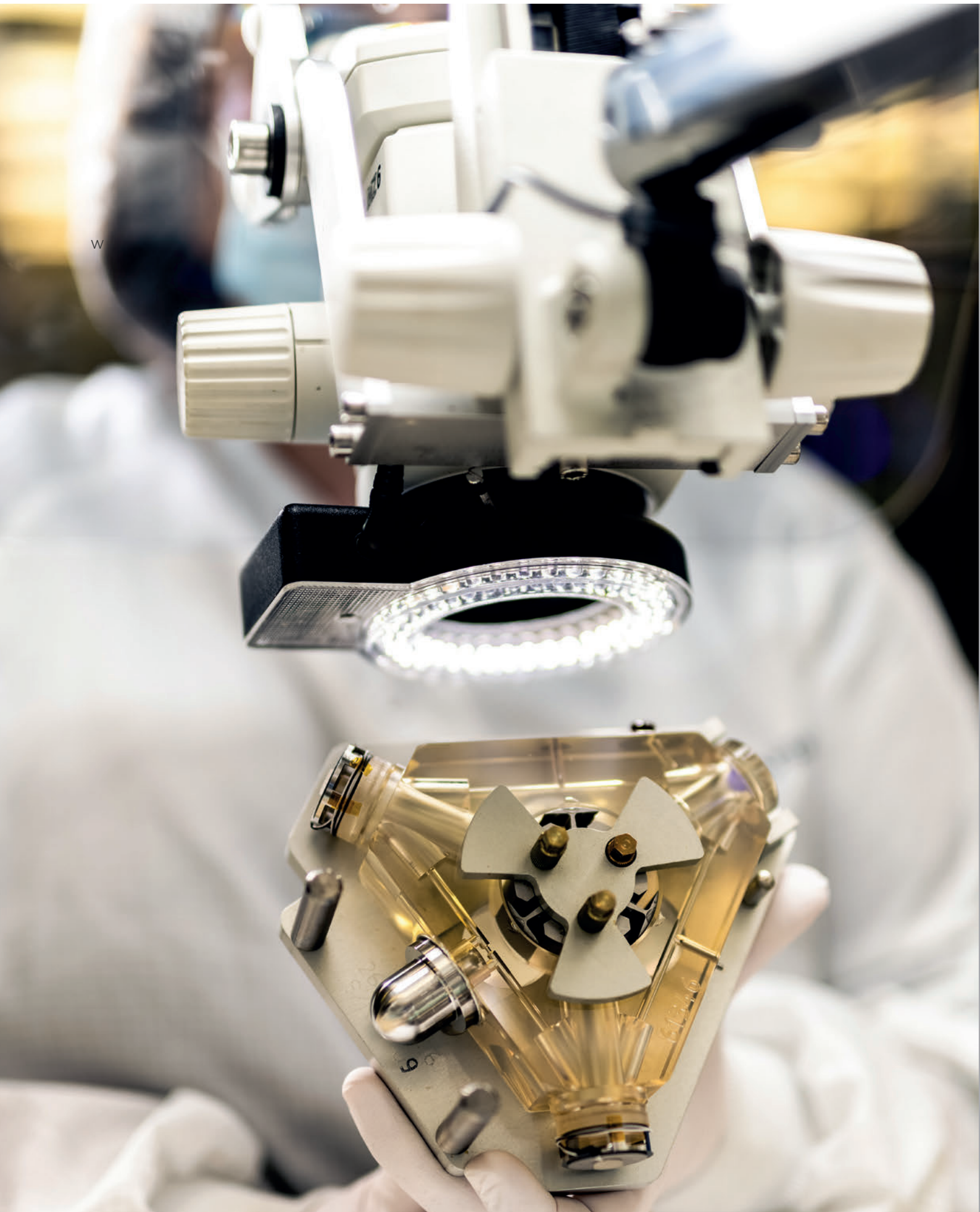
Integration on a ring laser gyroscope in a cleanroom
