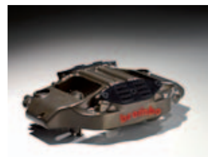
Brembo Racing. WRC caliper with liquid cooling.
