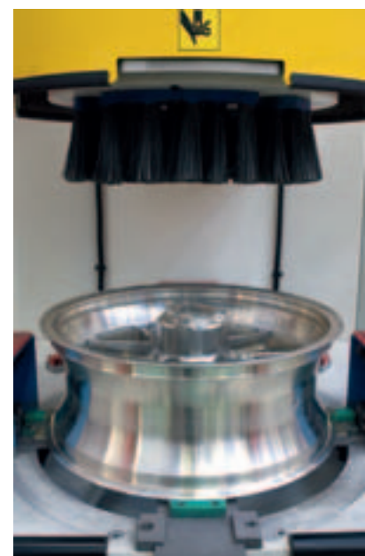
Performance Curno plant (Italy). Polishing machine for Marchesini motorbike rims.
