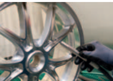
Curmo performance plant (Italy). Manual deburring of Marchesini rims.
