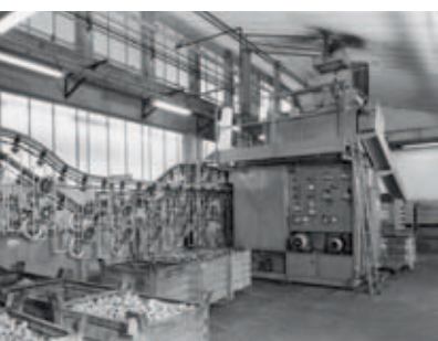
The lubrication and drying line for finished discs at the plant in San Giovanni Bianco (Bergamo), late Seventies.
