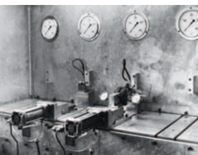
Test bench for checking the hydraulic tightness of calipers at the end of the assembly line at the plant in Paladina (Bergamo), 1973.
