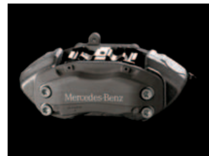
Cars. Aluminium and cast-iron fixed caliper, 1997.
