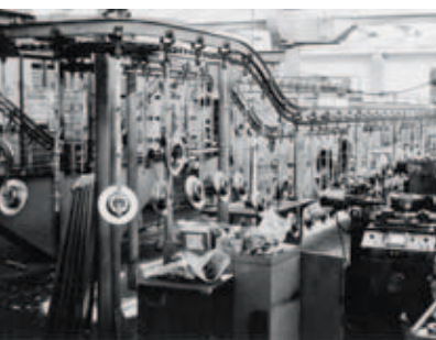
The lubrication and drying line for finished discs coming from the grinding machines at the plant in San Giovanni Bianco (Bergamo).
