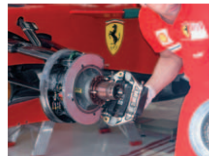
An assembly phase for a Formula 1 braking system.
