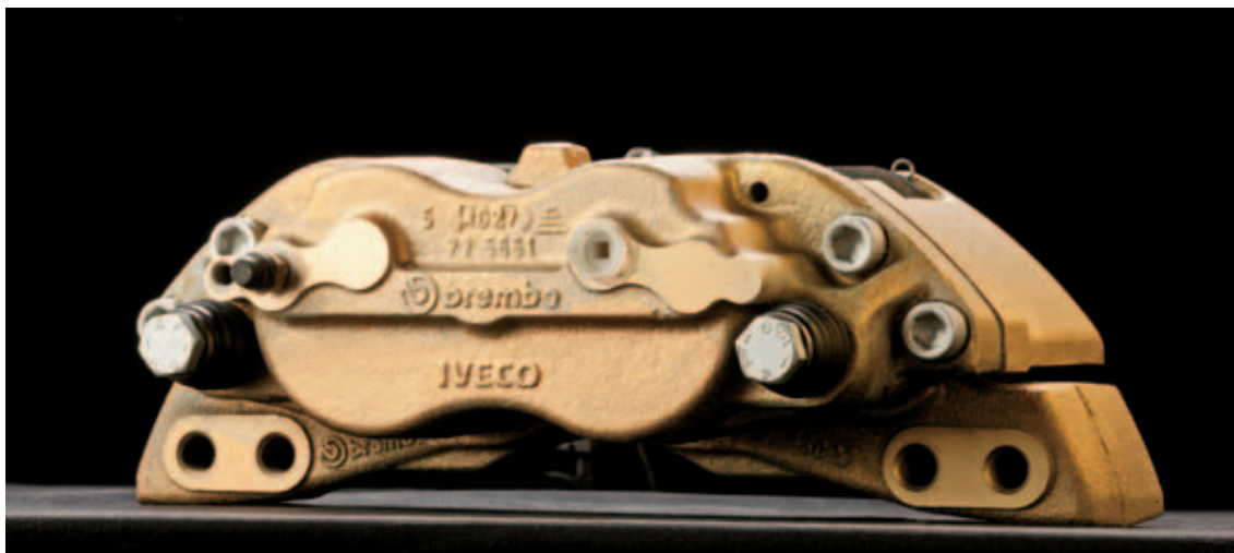
Commercial vehicles. Cast-iron floating front caliper, 1993.
