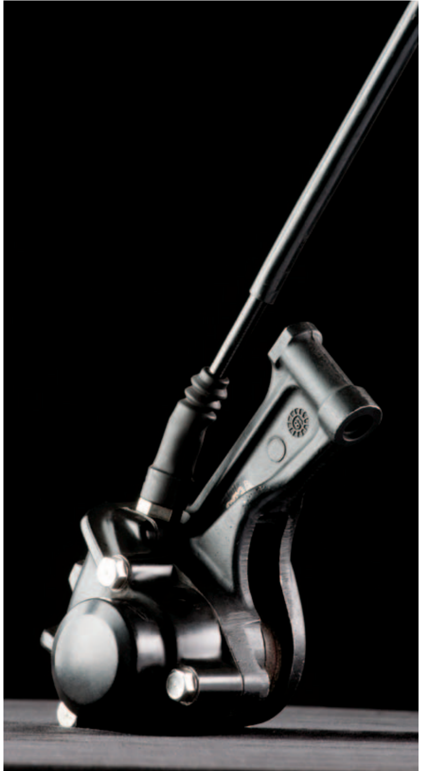
Motorbikes. Aluminium floating mechanical caliper, 1980.
