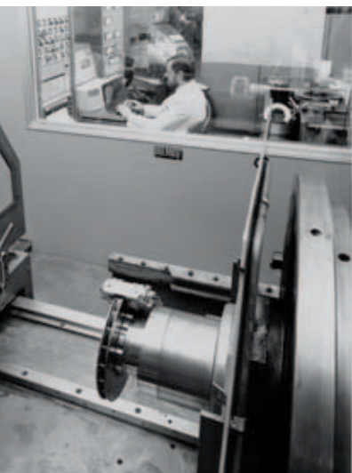
The first dynamic bench for testing discs at Paladina (Bergamo), 1982. A system for Formula 1 being tested on the bench.
