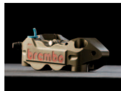
The first fixed monobloc caliper with radial fittings for the "500cc motorcycle Grand Prix", 1997.
