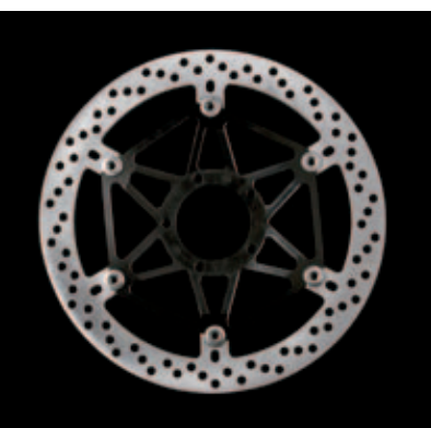
Floating disc for motorbikes, 2005. It features an aluminium hat and a stainless-steel braking surface to save on weight.
