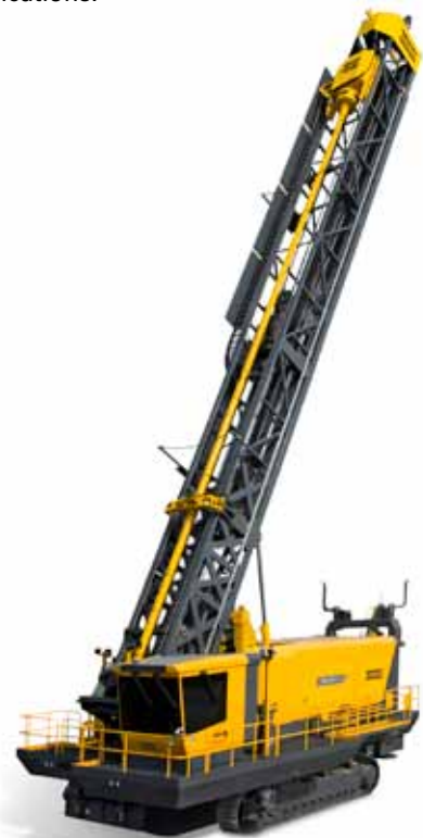
Rotary blast hole rig for open-pit mining
