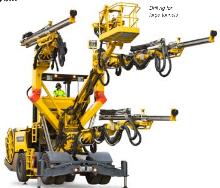
Drilling equipment increases drilling speed by up to 50%
