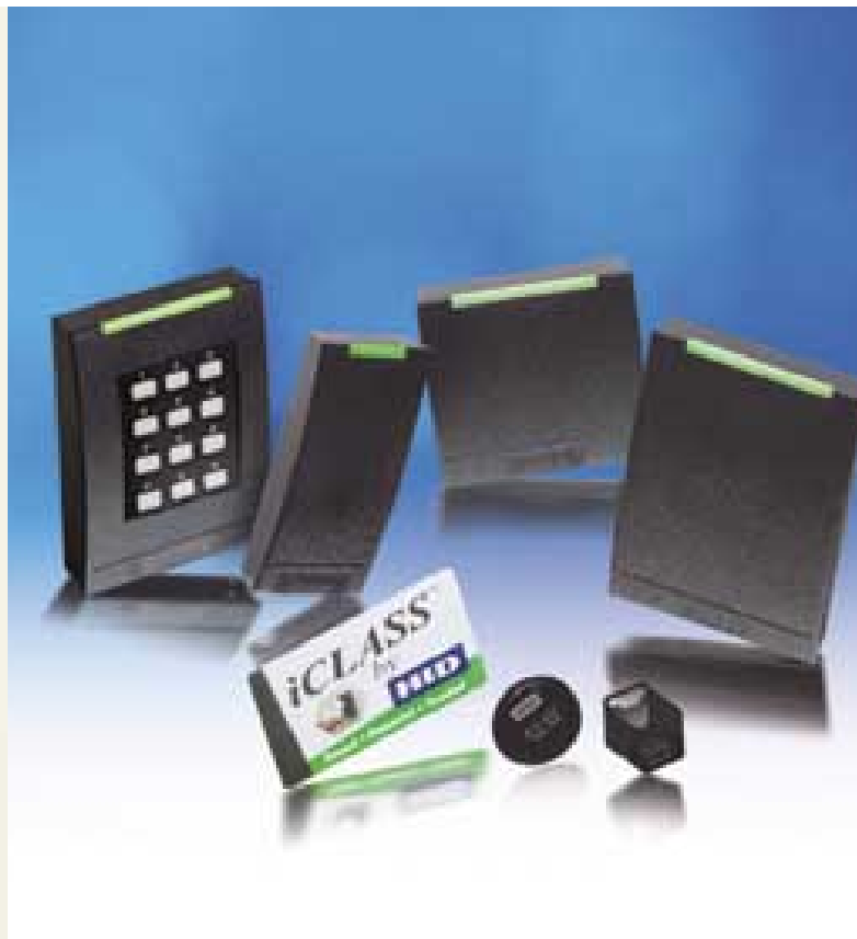
The iClass card combines RFID and a smart card.
